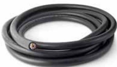
**SUBCAB® CABLES** are optimized for long-life submersible duty through their extremely low water absorption rates, superior mechanical strength and resistance to high temperatures and chemicals. Tight outer diameter tolerances ensure a reliable leak-free fit with the Flygt cable entry sleeve and built-in screened control cores secure proper monitoring and easy connection of pump sensors.
