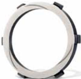
**ACTIVE SEAL™** technology from Flygt enhances sealing reliability by making the inner seal in a double seal system act as a micro pump. Laser-cut spiral grooves in the seal face of the inner seal pump liquid from the inner to the outer diameter of the seal ring, thus preventing liquid from entering the stator housing.
