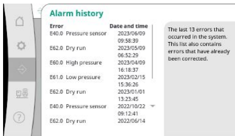
Fig. 57: Communication → Alarms → Alarm history menu item
