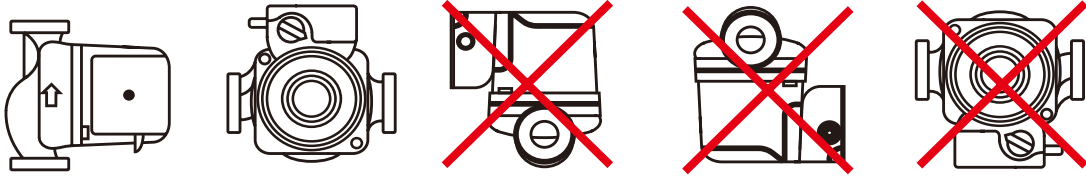
Fig2 installation position of electric pump
